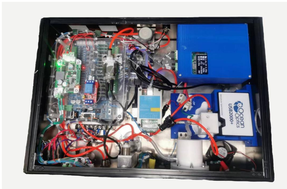
25 Fig S1. Photograph of direct sampling Hg analyzer. This instrument with 0.57 \times 0.42 \times 0.19 m dimensions, <12
