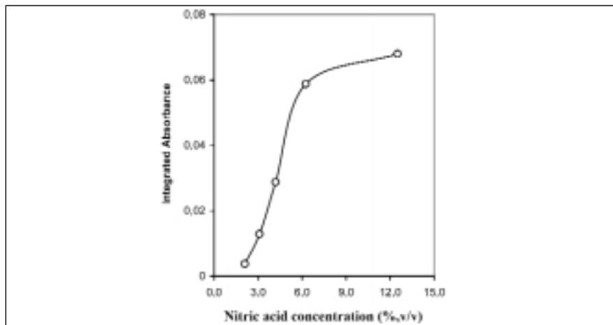
Fig. 5. Effects of eluent (nitric acid) concentration obtained at the following conditions:  $2.0 \mu\text{g L}^{-1} \text{Bi}^{3+}$ ; sample flow rate  $12 \mu\text{L s}^{-1}$ ; buffer pH 3.7; sample loading time 200 s; pyrolysis temperature  $400^\circ\text{C}$ ; and atomization temperature  $1200^\circ\text{C}$ .
