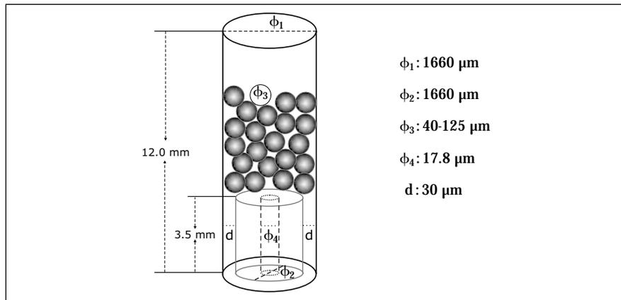
Fig. 2. Schematic diagram of the micro column.
