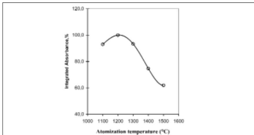
*Fig. 4. Effects of atomization temperature as obtained at the following conditions: 2.0 μg L<sup>-1</sup> Bi<sup>3+</sup>; sample flow rate 12 μL s<sup>-1</sup>; buffer pH 3.7; sample loading time, 200 s; pyrolysis temperature 400°C; and holding time 40 s.*
