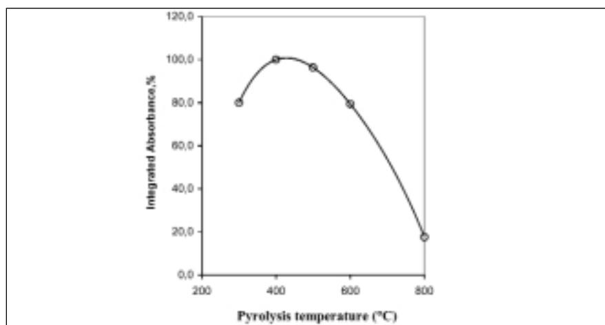
*Fig. 3. Effects of pyrolysis temperature as recorded at the following conditions: 2.0 μg L<sup>-1</sup> Bi<sup>3+</sup>; sample flow rate 12 μL s<sup>-1</sup>; buffer pH 3.7; sample loading time 200 s; holding time 40 s; and atomization temperature 1200°C.*
