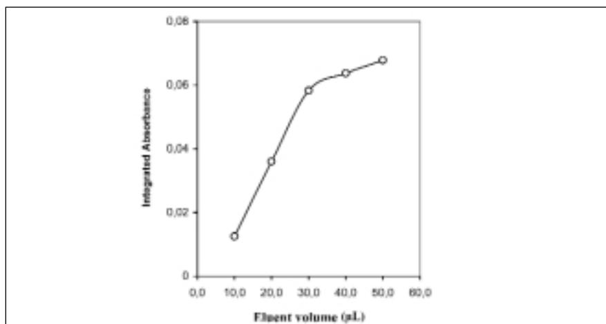
Fig. 6. Effects of eluent (nitric acid) volume obtained at the following conditions:  $2.0 \mu\text{g L}^{-1} \text{Bi}^{3+}$ ; sample flow rate  $12 \mu\text{L s}^{-1}$ ; buffer pH 3.7; sample loading time 200 s; pyrolysis temperature  $400^\circ\text{C}$ ; and atomization temperature  $1200^\circ\text{C}$ .
