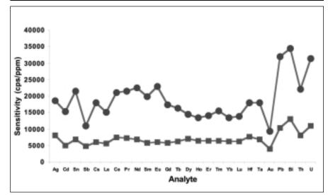
Fig. 4. Comparison of sensitivities measured in LA-ICP-SFMS with a plasma-shielded torch  $(\bullet)$  and without a shielded torch  $(\bullet)$  (GE –guard electrode) on NIST SRM glass 612 (rf-power: 1200 W; carrier gas flow rate: 1.35 L min<sup>-1</sup>).
