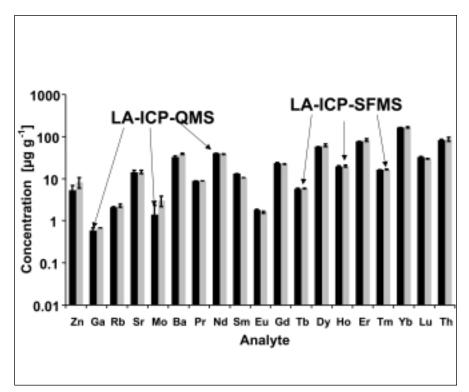
Fig. 5. Comparison of element concentrations in glass fibers measured by LA-ICP-QMS (left column: ELAN 6000, PerkinElmer SCIEX) in comparison to LA-ICP-SFMS (right column: Element, Finnigan MAT).
