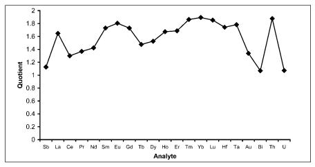
Fig. 2. Sensitivity measured on KL-2G (basaltic glass) divided by sensitivity measured on NIST SRM glass 612 using LA-ICP-SFMS.
