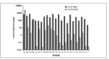
Fig. 3. Limits of detection on high-purity glass fibers in LA-ICP-QMS (ELAN 6000, PerkinElmer SCIEX) in comparison to LA-ICP-SFMS (Element, Finnigan MAT).
