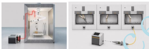
Fig. 3 (a) Schematic of the hot cell deployment configuration;(b) Conceptual deployment of the detachable FO-LIBS system for hot cells group applications.
